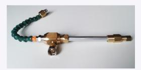
The TH series nozzles are expressly designed to obtain a significant thermal drop when the ambient temperature compressed air is canalized in the nozzle inlet and the temperature drop is obtained in the out coming compressed air (temperature decrease values between 15°C to 30°C depending from many factors, as inlet pressure and TH nozzle model).
